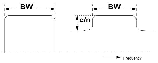
The left spectrum is showing a noiseless QPSK signal with BW (=bandwidth) symbol rate. The spectrum at the right hand side shows a real life situation with a certain Carrier to Noise ratio (C/N).
