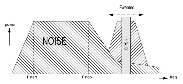
The noise spectrum to simulate 15 QPSK signals ranges from Fstart to Fstop, the wanted QPSK signal (Fwanted) can be set to each wanted frequency (in L-band). Also for the wanted frequency a certain C/N value can be adjusted.
